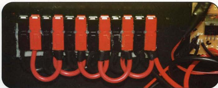
Photo 6. A daisy-chained panel fed from the master power switch was created. The panel was glued together and then mounted on a hook-and-loop fastener strip before being attached to the back of the toolbox.
