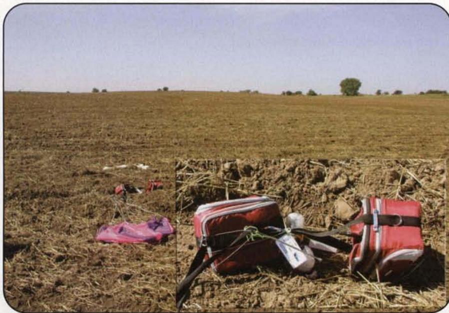
Enlarged view in the bottom right is of the payload containers and the load line knotted and tangled.
