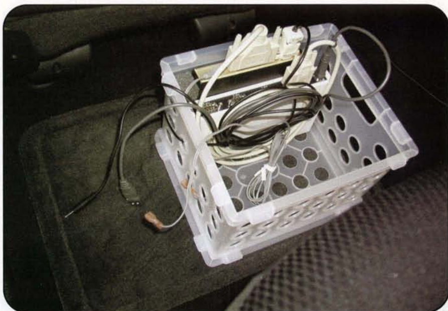
The tracking "crate" holding the Kantronics TNC and USB to serial adapter.
