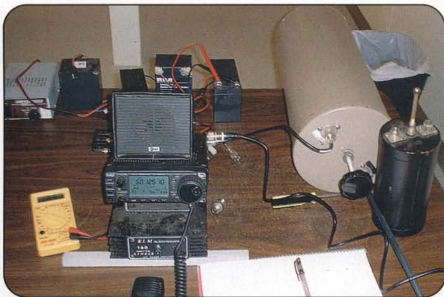
Photo 3. Cavity filter to the right of the transceiver.
