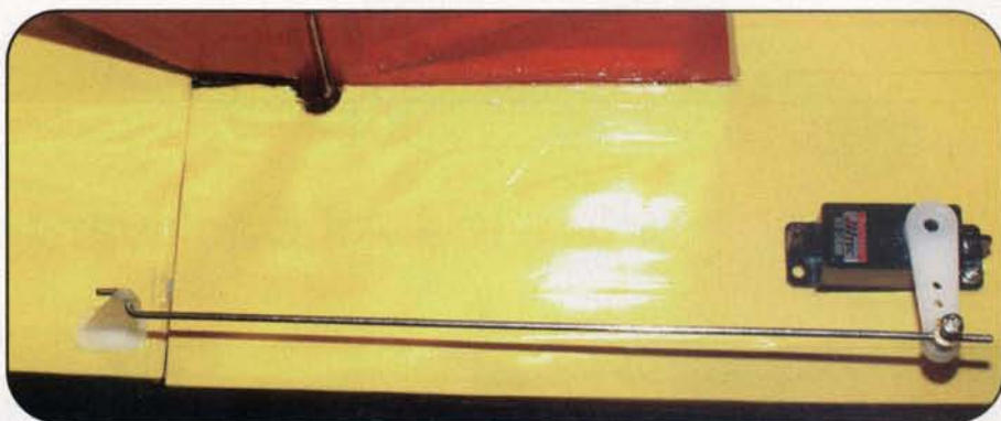
Rear-fuselage mounting of a rudder servo.
