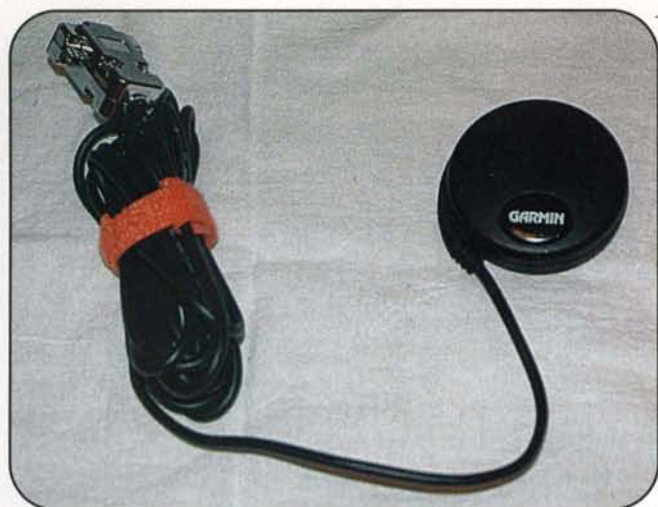
Photo 2. As a receiver for the tracker, the Garmin GPS-18LVC was chosen. It features bare-wire ends and gave the flexibility to create a customized connection that could also feed the sensor the power it needed.
