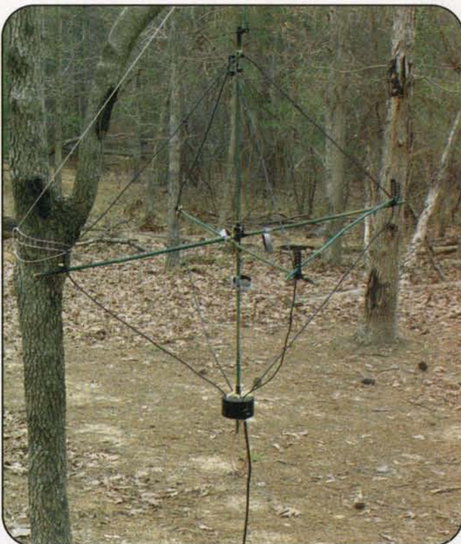
Horizontal polarization on 2 meters is standard at international ARDF events. Although "turnstile" crossed-dipole antennas are the most popular way to achieve an omnidirectional radiation pattern with horizontal polarization, Charles Scharlau, NZØI, used crossed-loop "eggbeater" antennas with equal success. (Photo by Joe Moell, KØOV)
