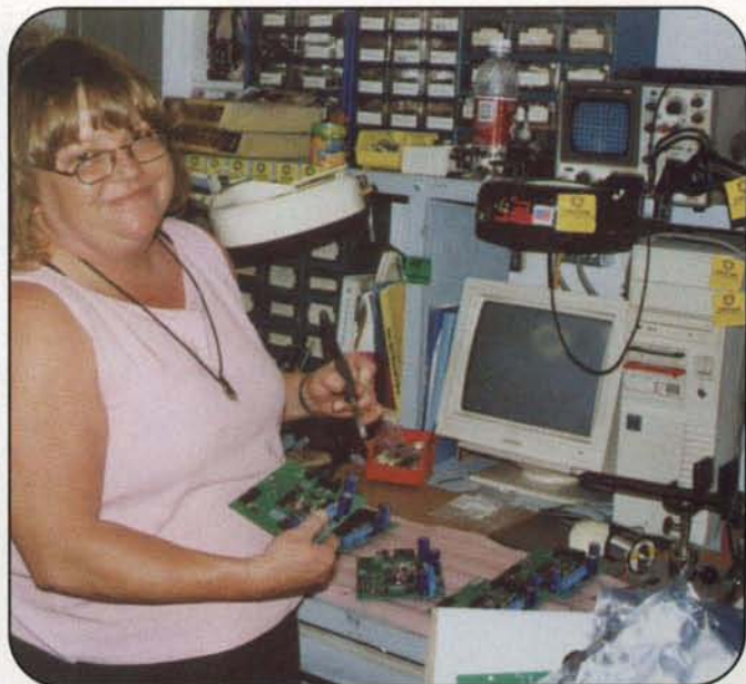
Robin does the final soldering on the RC2800 rotor controller board at M 2 .
